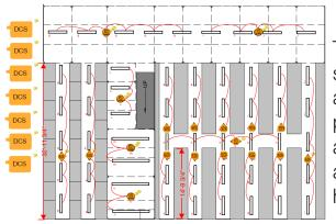
The IS 345 DCS sensors are field selectable for low or high bay applications. The IS 345 sensors work perfectly for data centers applications as the coverage pattern allows spacing and temperature rating to withstand the heat that radiates from the servers.
